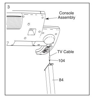
4. Insert the Console Wire Harness (78) and the TV cable into the Uprights (84).
